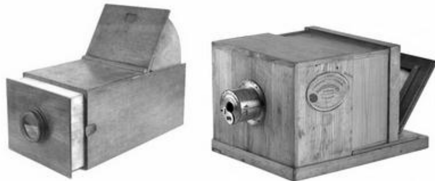
Left, Camera Obscura, c.1800. Right, Daguerreotype Camera, 1839.
